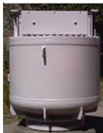
1965 First Voltage Transformer for SF6 insulated switchgear (GIS)
